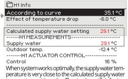
When system works optimally, the supply water temperature is very close to the calculated supply water temperature setting value. The circuit specific info view shows the temperature measu rements and the states of the actuators of the particular control circuit. (mo-
