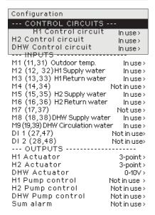
In Configuration menu the heating circuits and the inputs and outputs are configured and taken in use. The service code is needed for the access to the Configration menu.
