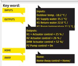
If a GSM is connected to the controller, you can read measurement information
