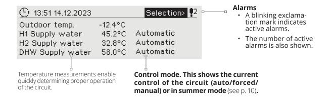
Acknowledging alarms: Press OK and the alarm sound will stop. If the reason for the alarm has not been corrected, the exclamation mark in the top right will continue to blink.
