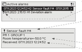
Every active alarm is shown in a separate row, where you can see when the alarm has become active. Press OK to get more information about the alarm.
