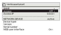
M-LINK supports Ouman Access-service which gives you a secure remote connection to the H23-device. With this setting you can activate the ACCESS-service in order to be able to use it. OUMAN ACCESS- service is "off" by default in H23.
