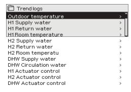
H23 controller automatically logs trend from the measurements. Select the measurement which log you want to view. The trend log will be shown in the controller's display. It's also possible to change the logging interval.
