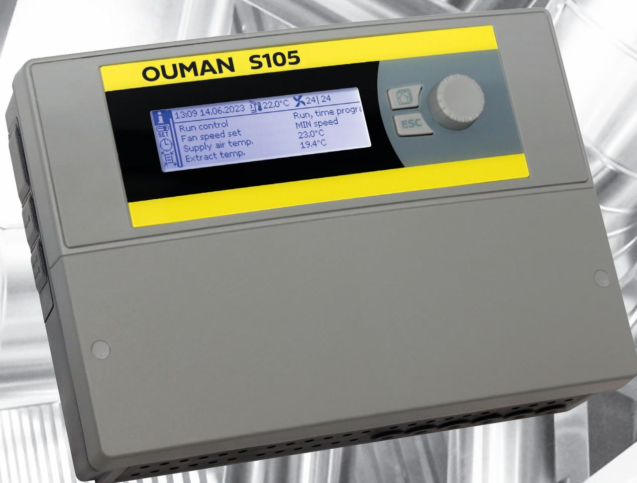
*The Ouman S105 is a compact and versatile air conditioning controller designed to manage 1-5 stage air conditioners: dampers, cooling, heat recovery, heating and fan controls. It is suitable for both stepless frequency converter-controlled and fixed-speed contactor-controlled AH devices, including AH devices with a battery.*
