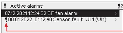
Every active alarm is shown in a separate row, where you can see when the alarm has become active. Press OK to get more information about the alarm.
