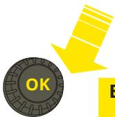
When the control knob is pressed down for an extended period of time, the hidden menus are displayed.
