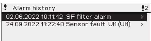
The reason, source and inactivation time (02.06.2022 10:11:42) is shown for every alarm in alarm history. The last 10 alarms can be seen in inactive alarms.
