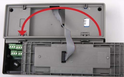
Turn the keyboard/display unit into the opposite position. Watch out for flat cable, that it does not shed.
