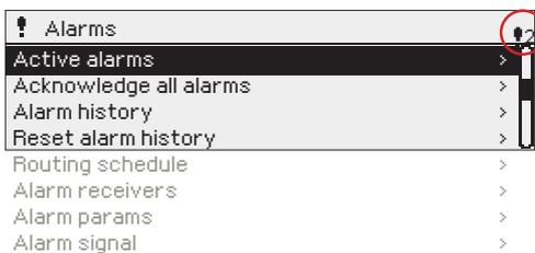
The alarm menu of the S105 device allows you to view both active alarms and previously active alarms. The number of active alarms is displayed in the top right corner of the main view.
