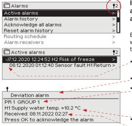
In the alarm menu of C203 device, you can check the active alarms and what alarms have been active. The number of active alarms can be shown in the main view if you wish.
