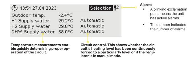
Acknowledging alarms: Press OK and the alarm sound will stop. If the reason for the alarm has not been corrected, the exclamation point in the top right will continue to blink.
