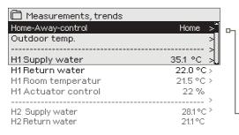
You can see the measurements and mode information linked to the C203. When you press OK on the measurement row, you can see the measurement's trend or trend log, change the settings of the trend log and change the name of the measurement.
