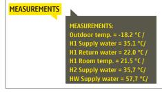
If a GSM is connected to the controller, you can read measurement information form a mobile phone.
