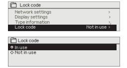
If you take lock code into use, you can read C203 device information when the device is locked, but you can not change settings. It is recommended, for example, that you take lock code into use if the device is located so that anyone could reach it and change settings (e.g. deactivate burglar monitoring). Locking the device and changing the lock code prevents unauthorized use of the device.
