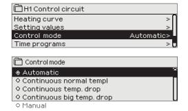
Automatic control is the mode that is used normally. You may change automatic control to manual control here, and drive the valve to the desired position. You can also force a mode to the desired temperature level. A continuous mode command bypasses possible scheduling programmes.
