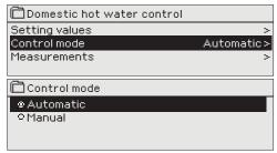
Automatic mode is normally used in regulating domestic hot water. Here you can switch from automatic to manual mode and move the valve into the desired position. You can use manual mode for example when a sensor malfunctions.
