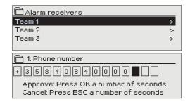
A GSM modem can be connected to the C203 unit to send information about the alarm as a text message to the alarm team. A substitute team can also be designated. The alarm is sent to the team that is set in the alarm system's software as the correct team for that time.
