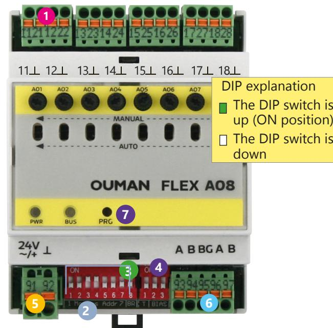
① Detachable spring loaded strip connectors (analog outputs)
