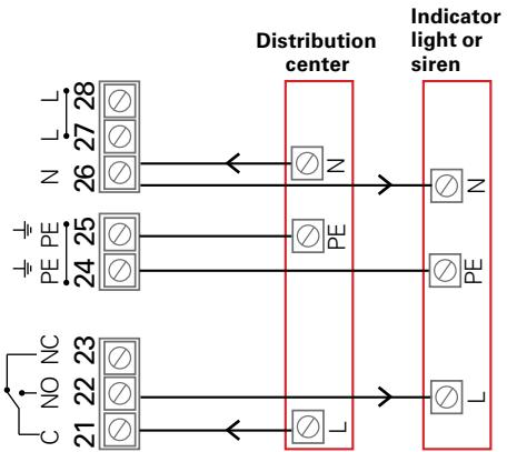
**Relay control according to the temperature and the relay controls the 230V device, for example, the cooler's fan**
