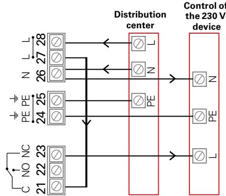
**Relay control is used for pump summer stop**
