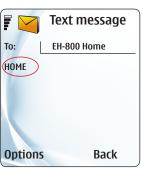
Use home control when a temperature drop has been made for the controller using the week/24 hour program or the exception calendar and you want to bypass the present temperature drop command. The home command switches the controller to a nominal temperature.
