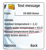
When either a "Home" or "Away" command is sent to the controller, the controller sends an informative OUMAN message as a return message. The message shows the temperature to which the Home/Away control (H-A) controls the controller.
