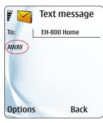
Use the away control command when you want to switch to a temperature drop. The controller maintains the temperature drop until it receives a "Home" control command. The control command can be given via a mobile phone, Home/ Away switch or from the controller. If the controller has an exception calendar program in use and a "Home" control command has taken it from use, an "Away" control command will return the exception calendar back into use.
