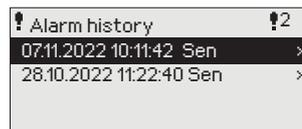
The reason, source and inactivation time (07.11.2022 10:11:42) is shown for every alarm in alarm history. The last 10 alarms can be seen in inactive alarms.
