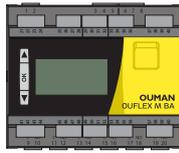
If you want to connect the Ouflex M BA unit to an Ethernet network, you will need an M-LINK adapter (additional equipment). M-LINK is connected to the COM3 port (RJ45) located on the side of the controller. The maximum length of the RJ45 ethernet cable between Ouflex M BA and M-LINK is 10m and all 4 pairs must be connected. If you have changed your network settings, select "Update Network Settings".
