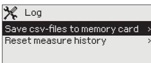
Ouflex M BA allows you to save CSV files to the memory card. Additionally, you can reset the measurement history directly from the device's internal memory.
