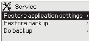
The "Restore Application Settings" function allows the device to revert to the settings it had when the existing application was first downloaded.
