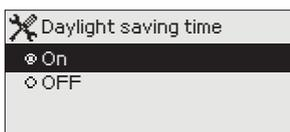
This setting is hidden setting. You can hide/show these settings by pressing OK for a few seconds. The controller will automatically be switched to daylight saving time and to standard time, if the selection "On" is made.
