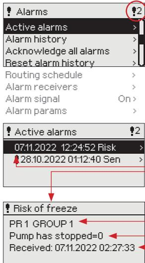
The alarm menu of the Ouflex M BA device allows you to view both active alarms and previously active alarms. The number of active alarms is displayed in the top right corner of the main view.
