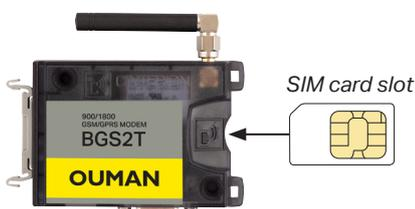
Set the SIM card to SIM-slot that is in the side of the modem, so that circuit of the SIM-card is facing towards the sticker that is on the top of the modem. Press the SIM-card until the slot snaps and card is properly attached to slot. The SIM-card can be removed by using a flat object such as a screwdriver with flat-head.
