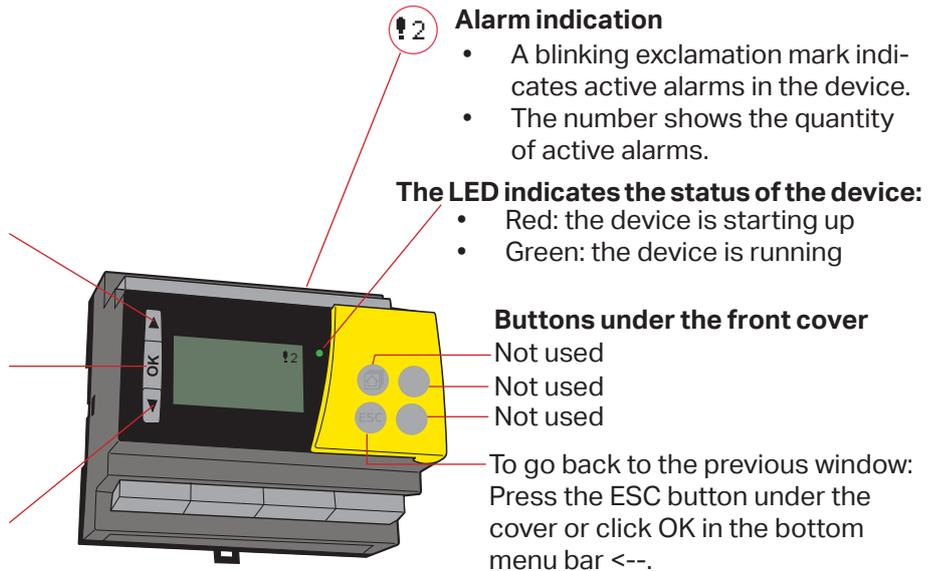
**Alarm acknowledgement:** press the OK button. The beeper will be turned off. If the cause of the failure is not fixed, the exclamation mark in the upper right corner of the display will keep blinking.
