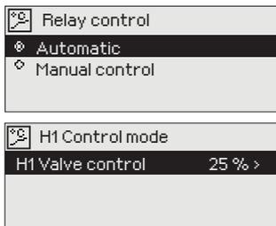
The default mode of operation for the controller is automatic control. However, if your application permits changing the control mode, you can switch from automatic control to manual control using this feature.
